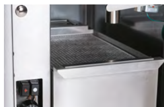
Oil drain into the container
