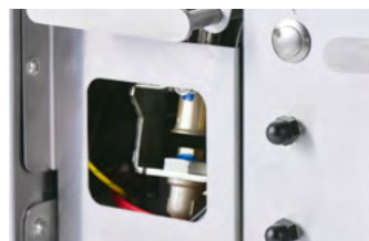
Spark generator supplied with 230 V
